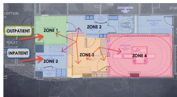
A very compact (and efficient) 4-Zone MRI suite plan
